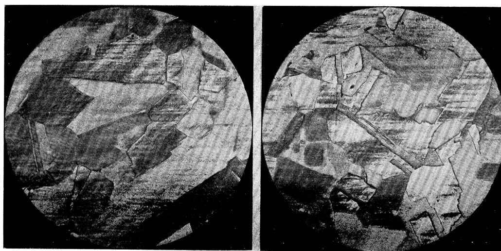
FIG. 4.—Specimen 1010. Manganese steel quenched from 1,000^{\circ} in water; the structure shows twinning and consists of austenitic grains. (a) Before immersion in liquid hydrogen; (b) after immersion.
